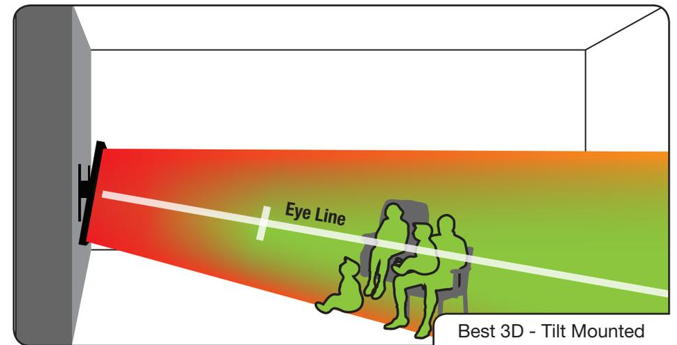
In this example, the viewers have mounted the TV on a **Tilt Mount**. They are at the correct distance and they are viewing the TV straight-on, close to the ideal eye line. They will experience good 3D picture quality.
